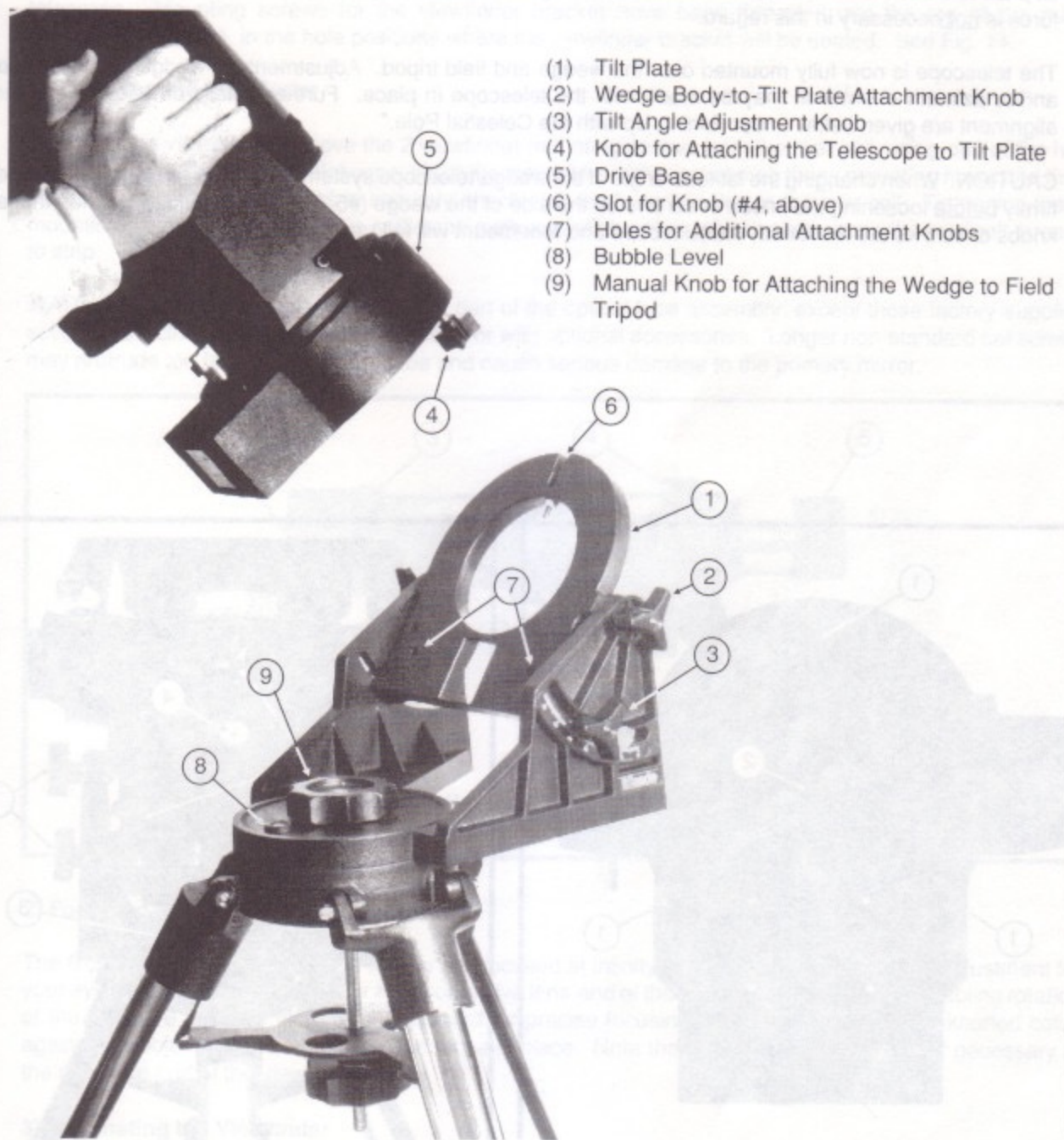
Fig. 11: Placing the Telescope on the Equatorial Wedge
