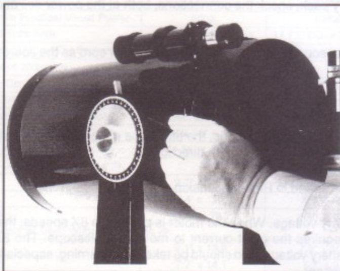
Fig. 33: Adjusting the Declination Lock.
