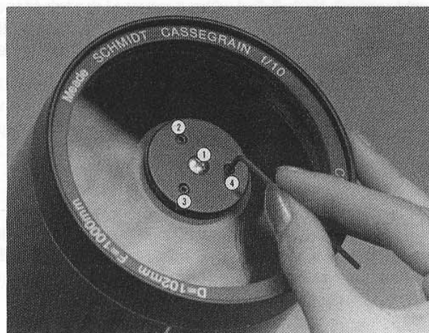
Fig. 3: Collimation of the Optical System
